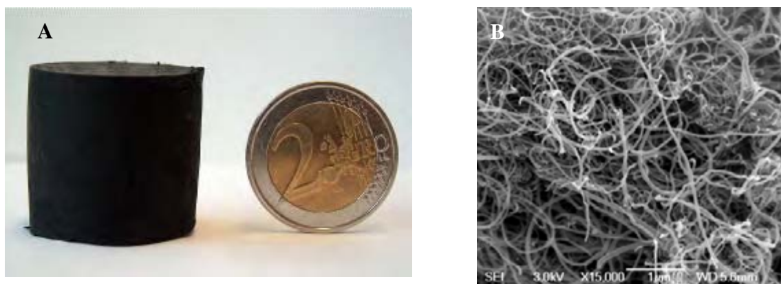
Figure 1: A. Picture of the self-supported MWNTs, B. SEM picture of self-supported MWNTs after \text{HNO}_3 and \text{NaOH} washing.
